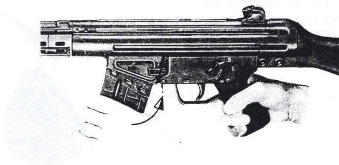
Fig. 53: Insertion of the magazine
