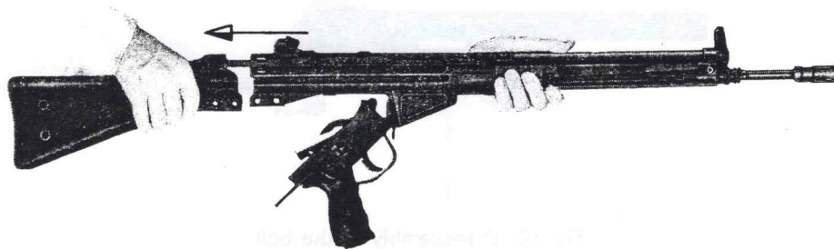
Fig. 63: Remove back plate with butt stock
