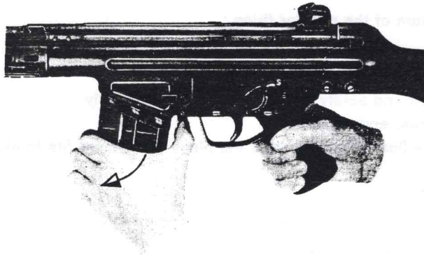
Fig. 54: Removal of magazine
