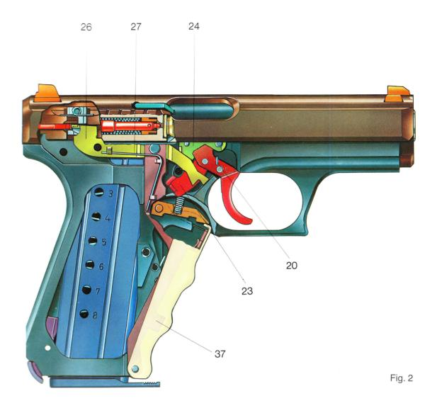
Pistol loaded and uncocked (Fig. 2).
