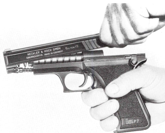
Fig. 11 Lift slide off
