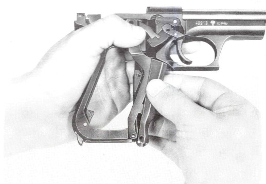
Fig. 21 Mounting the squeeze cocker
