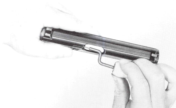
Fig. 14 Inserting of spring pin
