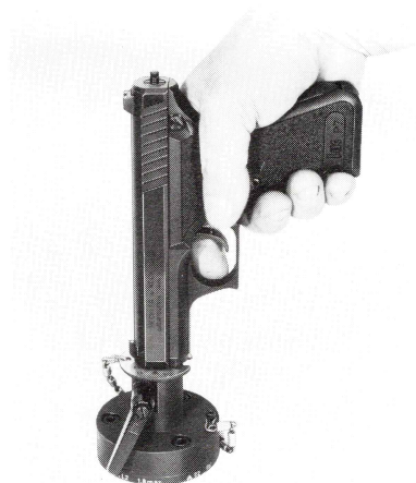
Fig. 5 Depressing the pistol onto the gauge
