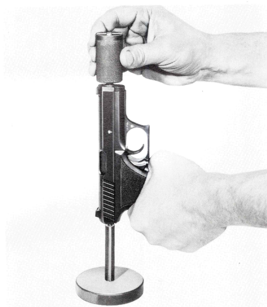
Fig. 8 Introduce depth gauge
