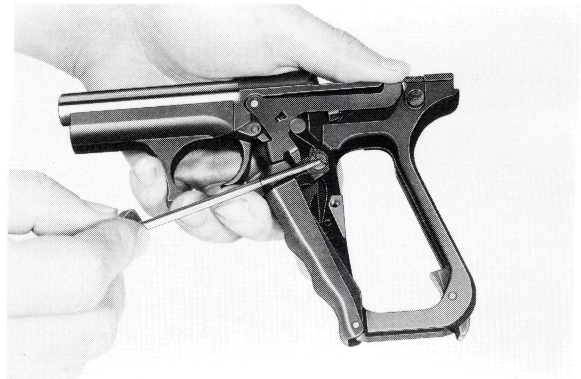
Fig. 17 Engaging rocker spring
