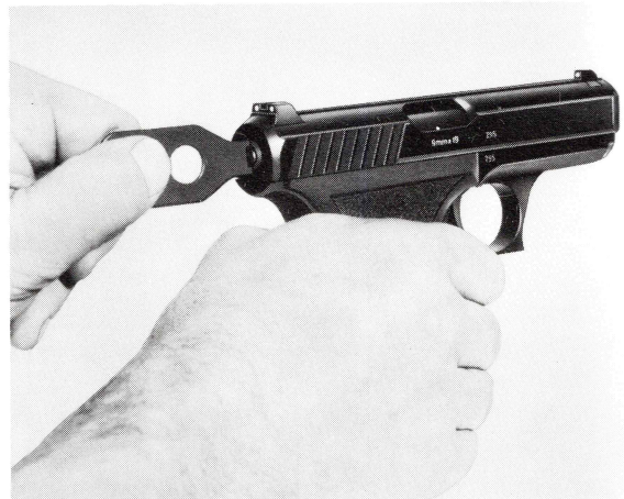
Fig. 9 Press firing bushing forward
