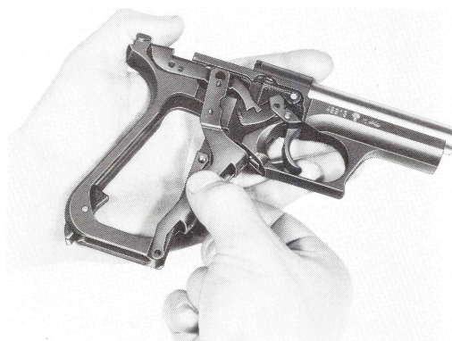
Fig. 20 Mounting the drag lever
