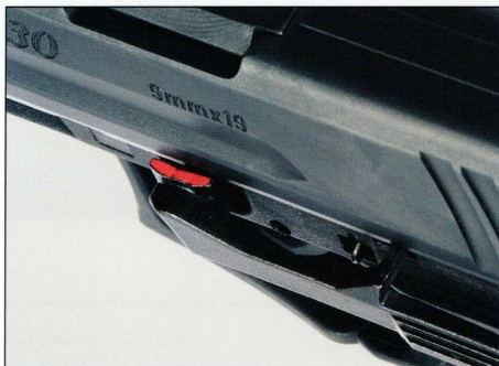
Slide release Retains slide for easy field stripping
