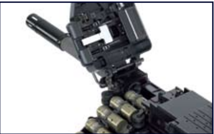
FEED SYSTEM Driven by the bolt, the system feeds and guides the linked cartridges in two smooth movements during the forward and rearward movement of the bolt. The feed direction can be readily reconfigured from the right-side to left-side by the operator in the field in minutes, without the use of tools.
