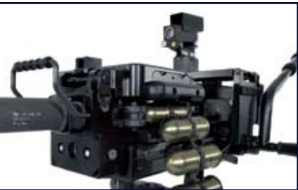
FEED SYSTEM Driven by the bolt, the system feeds and guides the linked cartridges in two smooth movements during the forward and rearward movement of the bolt. The feed direction can be readily reconfigured from the right-side to left-side by the operator in the field in minutes, without the use of tools.
