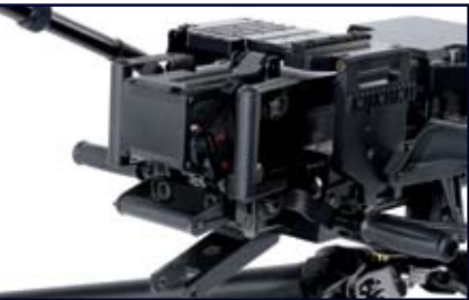
OPERATING ELEMENTS The safety/fire lever selector, trigger, and the charging handle are all located centrally on the end to the receivers
