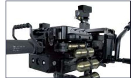
A robust, recoil operated inertia bolt with advanced primer ignition, firing from an open bolt position, directly chambers the cartridges out of the belt. The bolt fires all types of available 40 x 53mm grenades in either semi or fully automatic firing modes. Semi-automatic fire increases hits of target while reducing rounds fired.
