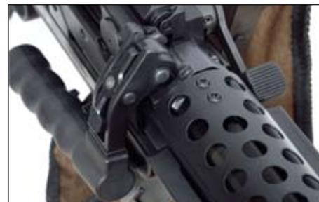
**SAFE BARREL LOCK, QUICK BARREL CHANGE**
