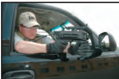
HK grenade launchers can be fired without a stock using a special bungee sling.
