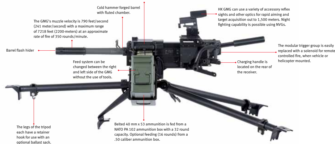
UPPER MOUNT (GUN CRADLE) The upper mount/gun cradle effectively buffers recoil using twin hydraulic buffers and includes handles, a secondary trigger lever, a shoulder support rod, MIL-STD-1913 Picatinny attachment points at the 3, 9, and 12 o'clock positions for mounting optional sighting systems, and the mounting for the ammunition box. The GMG receiver assembly is easily installed into the upper mount/gun cradle in seconds without tools. FEED SYSTEM Driven by the bolt, the system feeds and guides the linked cartridges in two smooth movements during the forward and rearward movement of the bolt. The feed direction can be readily reconfigured from the right-side to left-side by the operator in the field in minutes, without the use of tools. A robust, recoil operated inertia bolt with advanced primer ignition, firing from an open bolt position, directly chambers the cartridges out of the belt. The bolt fires all types of available 40 x 53mm grenades in either semi or fully automatic firing modes. Semi-automatic fire increases hits of target while reducing rounds fired.
