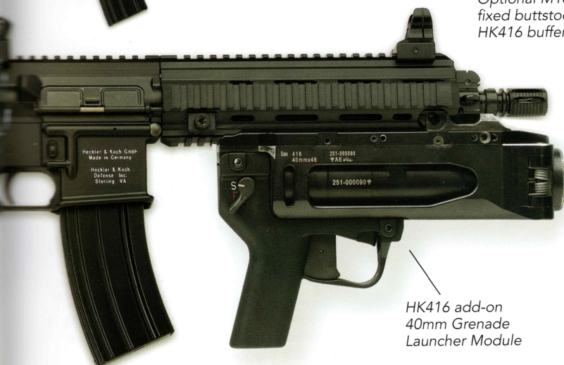
HK416 5.56mm Carbine Model D145RS with 14.5 inch barrel
