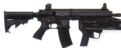
HK416 model D10RS with HK AG416 40x46mm add-on grenade launcher.
