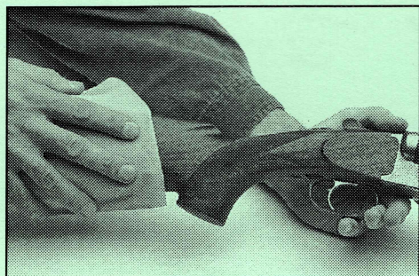
(figure 21) Stock being cleaned with cloth
