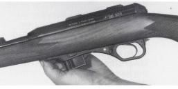
Note: When depressing the catch lever, always let the bolt travel forward freely, under its own inertia.
