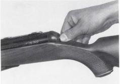
Remove the retaining pin.
