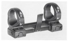
Our HK 05 clamp mount readily accepts standard telescopic sights adjustable for windage and elevation. If a telescopic sight with mounting rail is to be used, loosen the two hexagon socket screws on the bottom of the 05 clamp mount, slide on the telescopic sight and tighten both hexagon socket screws firmly. For telescopic sights without mounting rail, the clamping rings must be used additionally.
