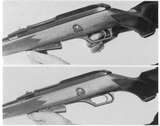
Then retract the bolt all the way by means of the cocking lever on the right side of the rifle. The catch lever located behind the cocking lever will engage and hold the bolt open. Depressing the catch lever slightly will cause the bolt to snap forward, chamber a round from the magazine, and lock into the receiver. The rifle is now
