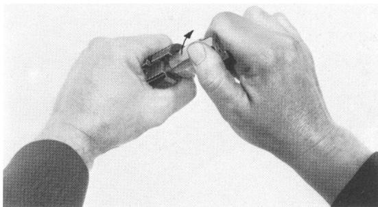
Rotate the bolt head clockwise one quarterturn, and then remove it from the locking piece. Finally, remove locking piece, firing pin and firing pin spring from the bolt head carrier by rotating the locking piece further
