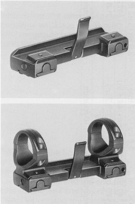
Our HK05 clamp mount readily accepts all standard telescopic sights. Should you wish to use an aluminum rail-type telescopic sight, loosen the two hexagon socket screws on the bottom of the 05 clamp mount, slide on the telescopic sight and tighten the two hexagon socket screws firmly at the rails. If you are using a steel telescopic sight, please also use the retaining rings.
