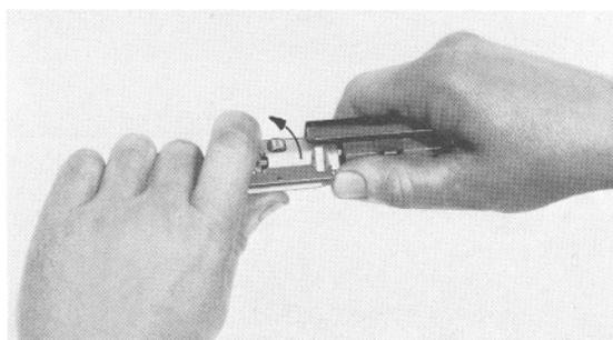
Place the bevelled surface of the bolt head beneath the spring-loaded bolt head locking lever. Strike the end of the bolt head lightly with the palm of your hand to force the bolt head far enough under the bolt head locking lever to provide a clearance of 3 mm (.12 in) between the bolt head and the bolt head carrier.
