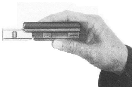
Then rotate the bolt head counterclockwise about one half turn, until the bolt rollers and the camways in the bolt head carrier are located at the same level. Then pull the bolt head away from bolt head carrier as far as it will go, so that the rollers recess com-
