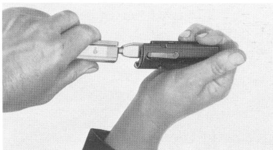
To assemble the bolt, proceed in the reverse sequence. First slide the firing pin spring onto the firing pin and insert both into the bolt assembly. Then press the locking piece against the firing pin spring and rotate counterclockwise one quarter turn. Assemble bolt head and locking piece as follows:
