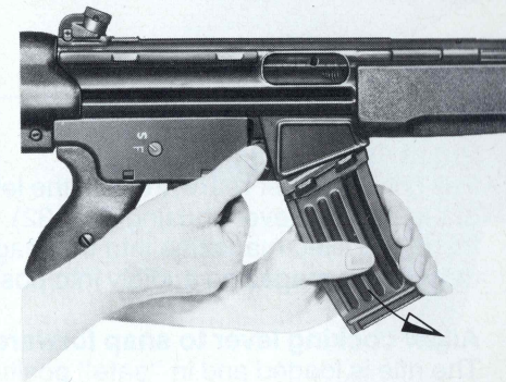
Fig. 31 Removing the magazine
