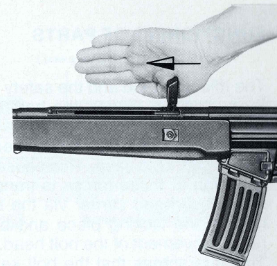
Fig. 33 Releasing the cocking lever
