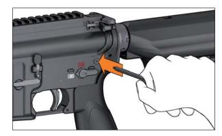
Fig. 43a: Pressing rear locking pin in to the right
