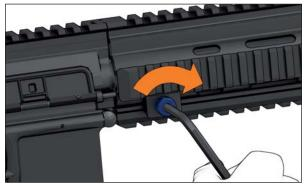
Fig. 55a: Tightening locking screw for handquard
