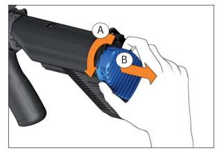
Fig. 28a: Removing buttstock cap
