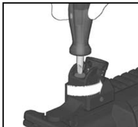
Fig. 8 – Clamping Screw (to tighten turn clockwise)
