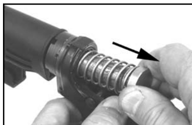
Fig. C – Removing non-HK Buffer and Action (Recoil) Spring
