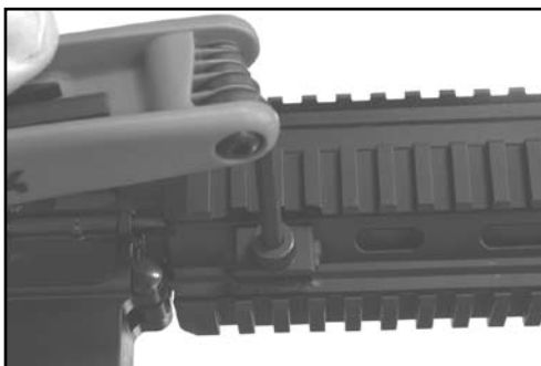
Fig. 44 – Loosening the FFRS screw with hex (Allen) wrench
