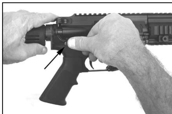
Fig. 7 – Completing the installation of the MR556A1 Upper Receiver on the Lower Receiver
