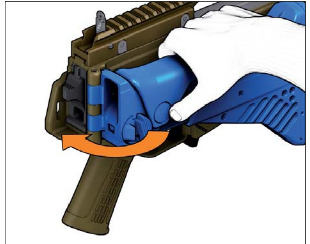
Fig. 25a: Unfolding the buttstock
