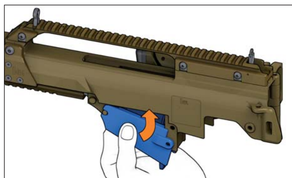
Fig. 46c: Swivelling the magazine well upwards
