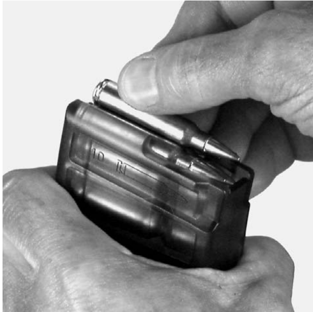
Fig. 19 Filling of magazine
