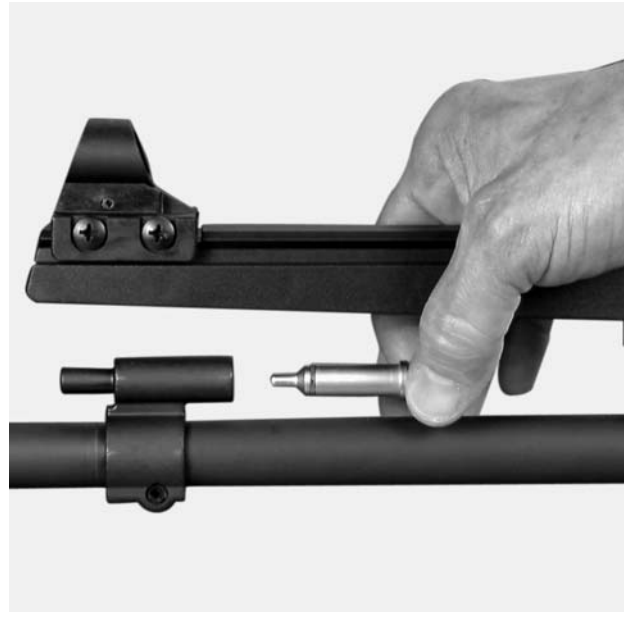
Fig. 29 Removal of gas piston
