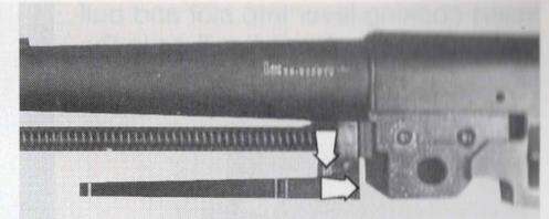
Introduce bolt head into bolt head carrier.
