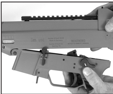
Fig. 23 Detaching lower receiver
