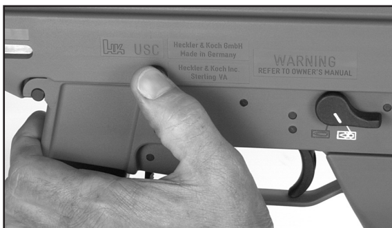
Fig. 21 Depress bolt catch to release the bolt
