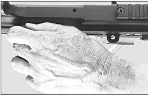
Fig. 20 Pull cocking lever backwards
