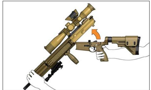
Fig. 68b: Assembling lower receiver and upper receiver
