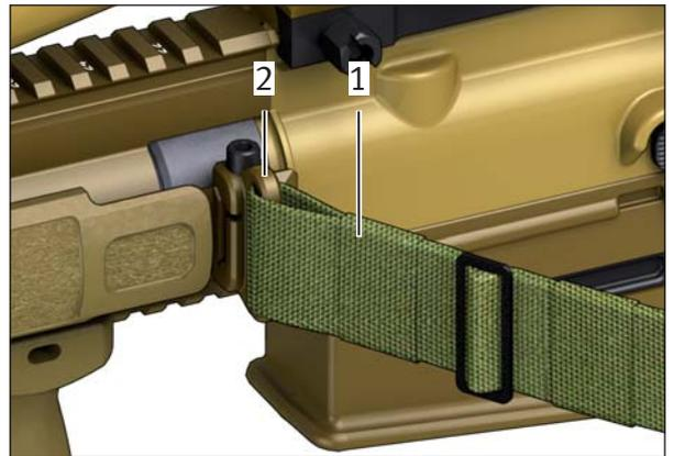
Fig. 33a: Attaching the carrying sling
