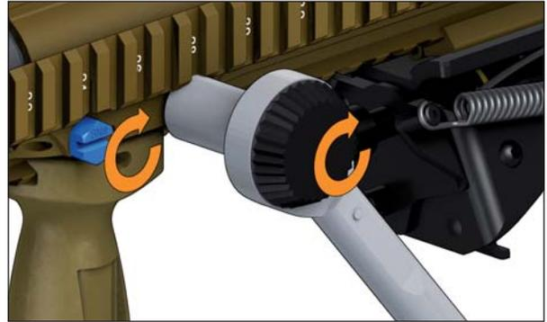
Fig. 67a: Tightening locking screws for handguard
