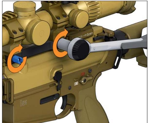
Fig. 69a: Tightening the screws of the telescopic sight mount with torque wrench
