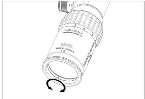
Fig. 85a: Adjusting the ocular
