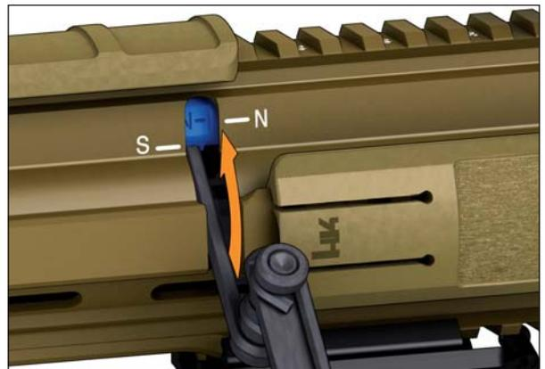
Fig. 37a: Rotating the adjustable gas nozzle
