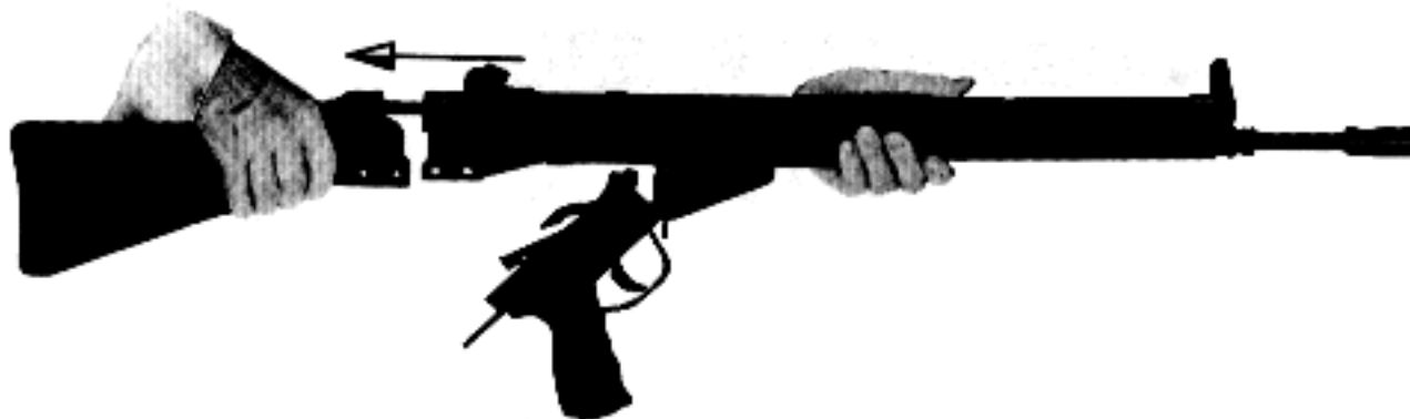
Fig. 63: Remove back plate with butt stock
