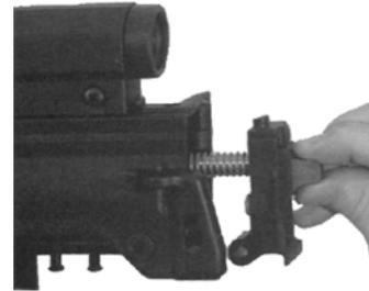
Fig. 37: Remove backplate
