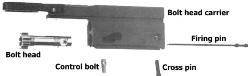
Fig. 41: Bolt, disassembled
