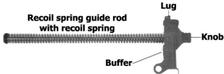
Fig. 13: Backplate with recoil spring.
