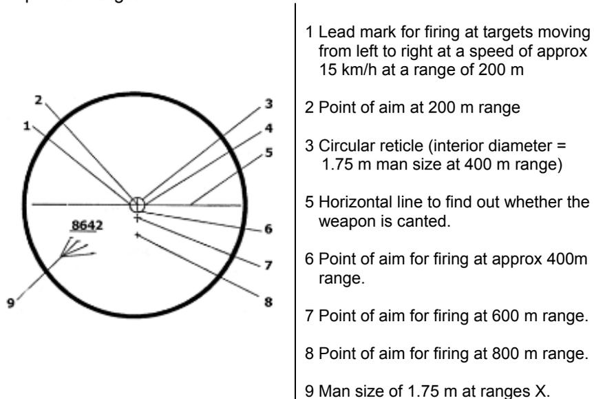
Fig. 47: Reticle of the optical sight
