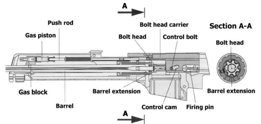
Fig. 32: Bolt, unlocked
