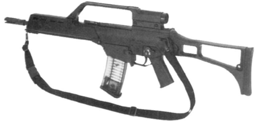
Fig. 3: G36K E Rifle with carrying handle, left side view.
