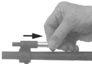
Fig. 40: Take out the gas piston
