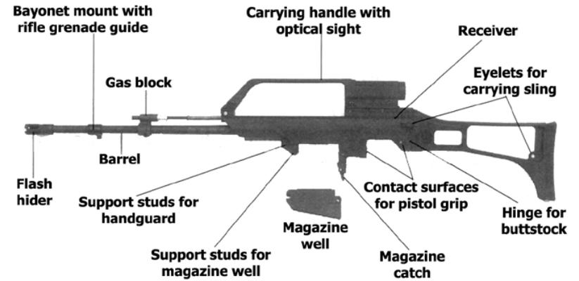
Fig. 8: Receiver with barrel, buttstock and attaching parts.
