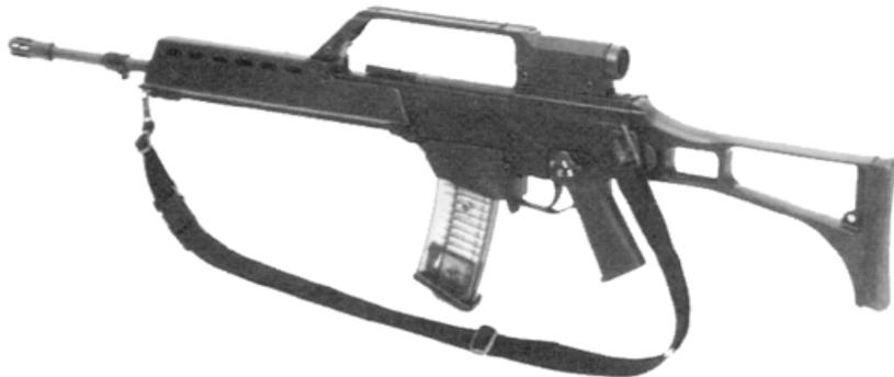
Fig.1: G36 E Rifle with carrying handle, left side view.
