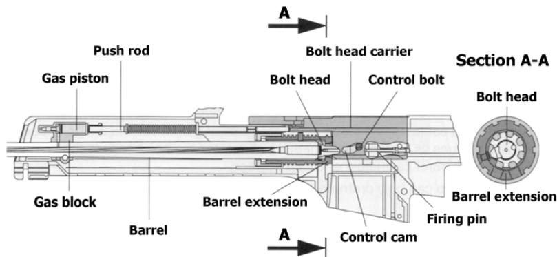
Fig. 31: Bolt, locked
