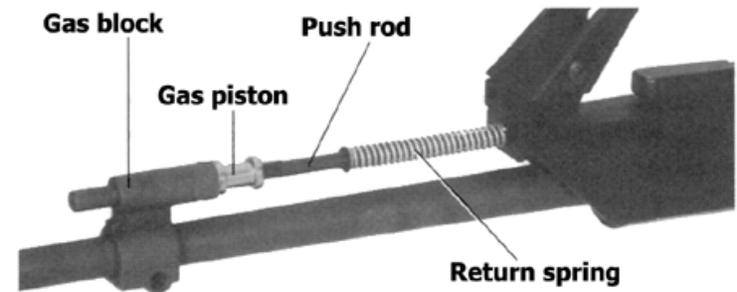
Fig.9: Gas operation assembly
