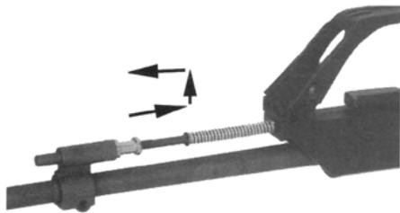
Fig. 39: Remove the push rod
