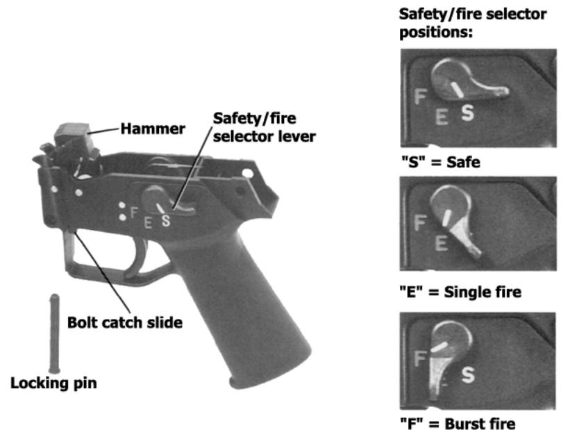
Fig. 14: Pistol grip with trigger mechanism
