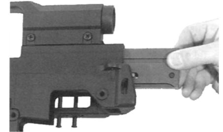
Fig. 38: Remove bolt assembly
