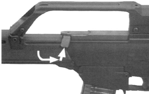
Fig. 36: Push on cocking lever (forward assist)
