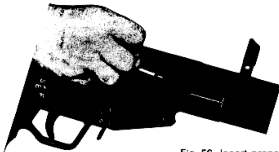
Fig. 56: Insert propellant charge
