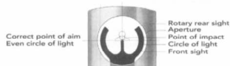
Fig. 74 Correct position of the front sight
