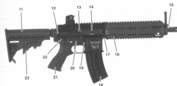
Fig. 2: HK416D10RS with HK diopter rear sight and MP5 type flip-up front sight, operating controls, right side view
