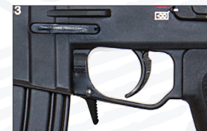
G36 magazine release lever
