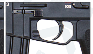
HK416/AR-15 magazine release lever
