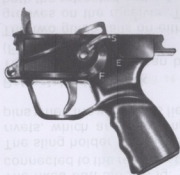
Fig. 12 Pistol grip with trigger mechanism
