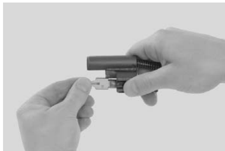
Fig. 21: Removing the bolt assembly components; stripping the bolt assembly
