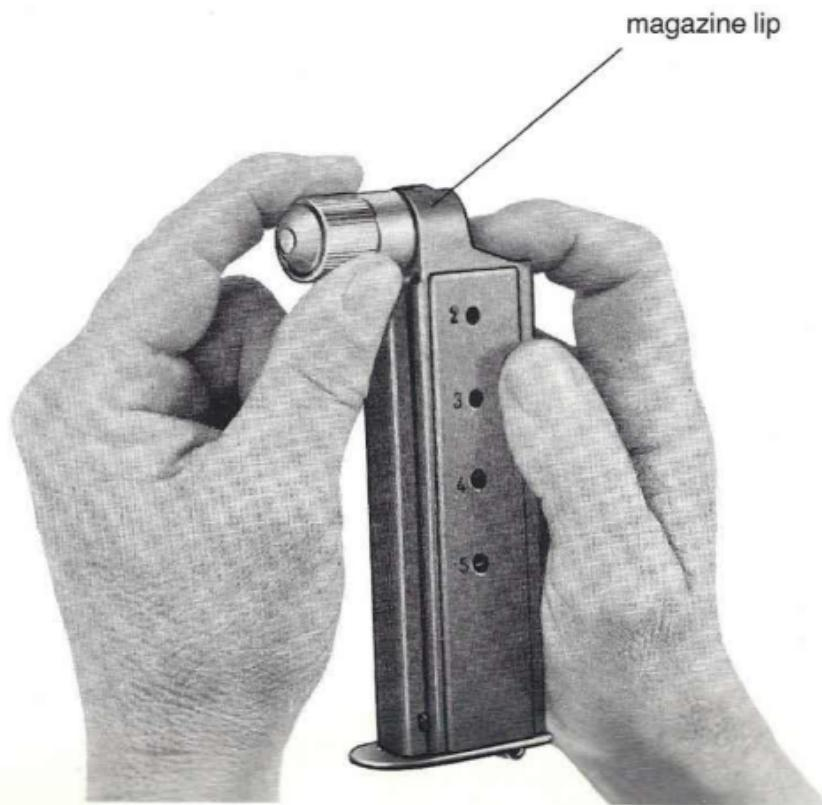
Fig. 4: Filling the magazine
