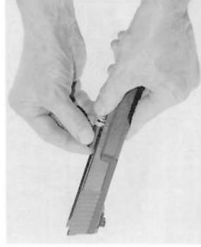
Insert the barrel into the slide and press backwards until it locks with the slide.
