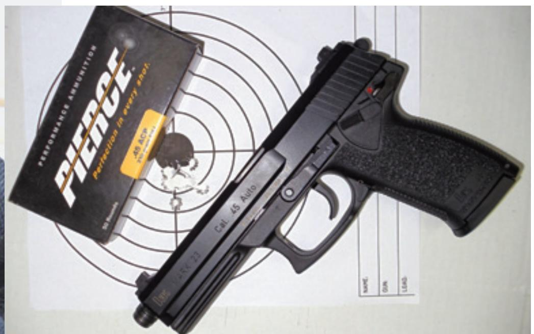
conditions a SEAL would encounter in his mission. This finish is a three step process beginning with the bare slide being nitro-carborised, second phosphate and coating of the black lacquer to give it the black appearance. Even if the black surface finish is worn off, the slide is still protected.
