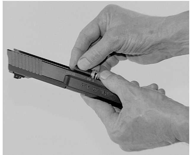
Insert the recoil/buffer spring guide rod
