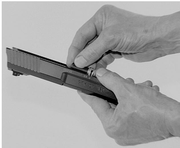
Insert the recoil/buffer spring guide rod
