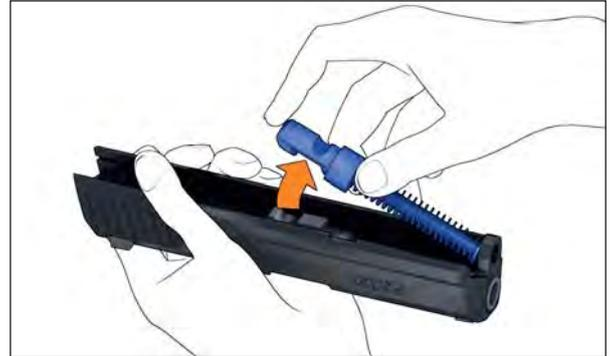
Fig. 41b: Removing recoil spring
