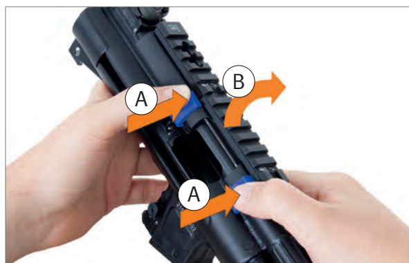
Fig. 29: Remove adapter with Picatinny rail
