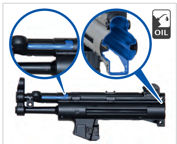
Fig. 33: Lubrication points of functional elements
