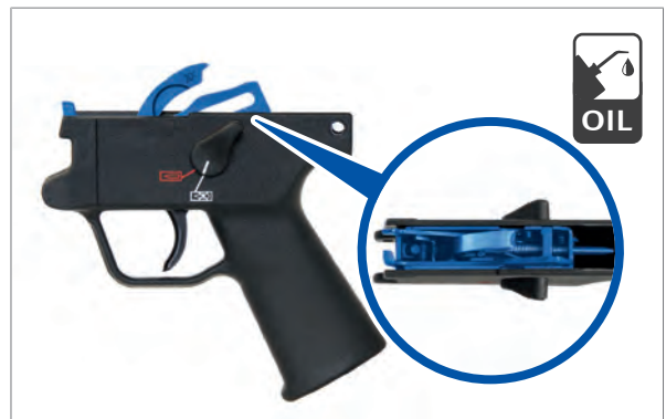
Fig. 32: Lubrication points on pistol grip
