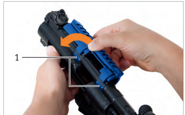
Fig. 34: Assemble adapter with Picatinny rail
