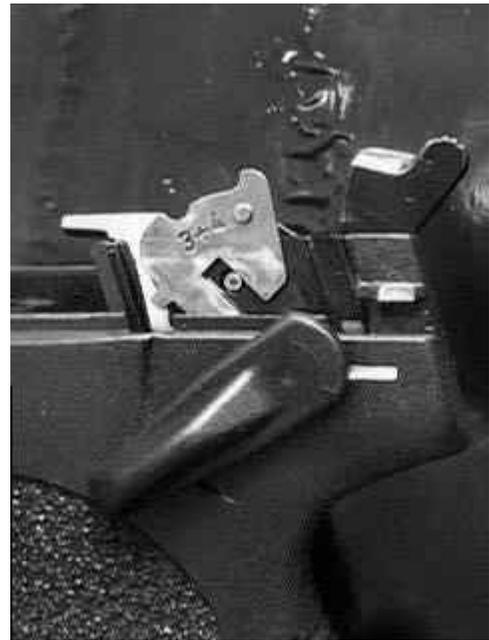
**Detent Plate almost completely removed**
