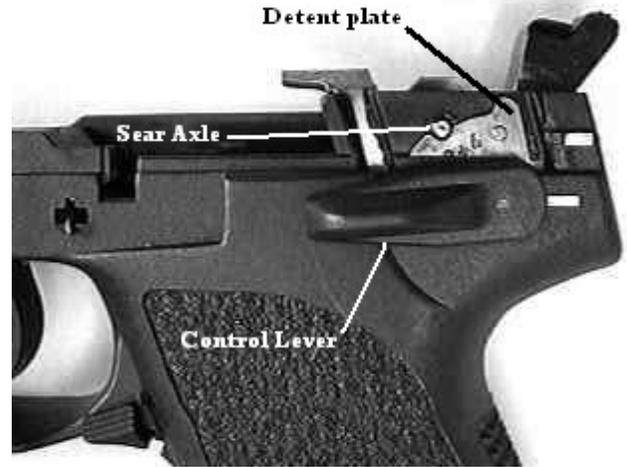
**Detail of Detent Plate and Sear Axle in final position**
