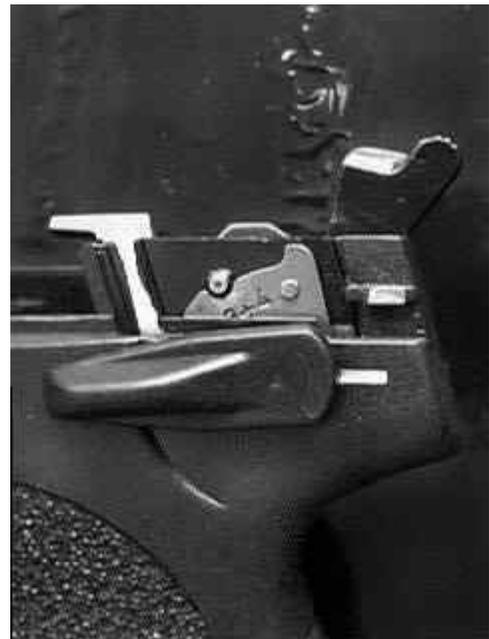
**View of Sear Axle, Detent Plate, and Control Lever**
