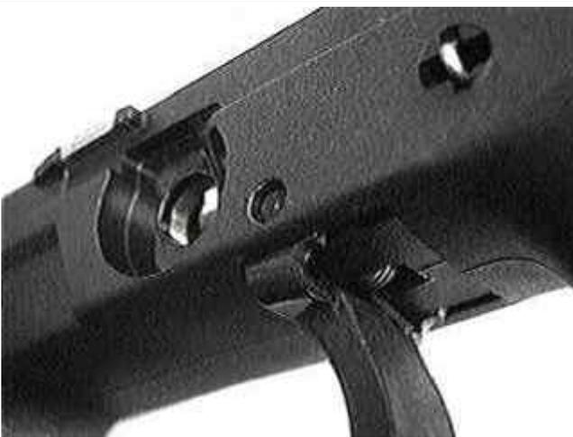
Detail of Trigger group when viewed from below (note rearward spring end is on back of Trigger)
