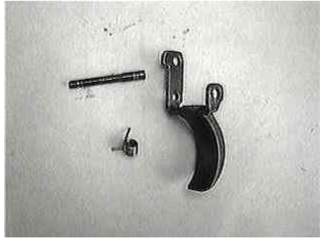
**Detail of the Trigger, Trigger Spring, and Trigger Axle removed**
