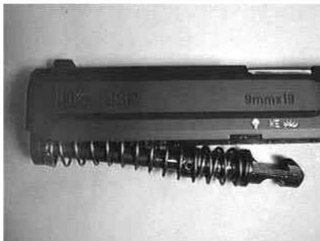
**Detail of installing the Recoil/Buffer Spring Assembly into the Slide**
