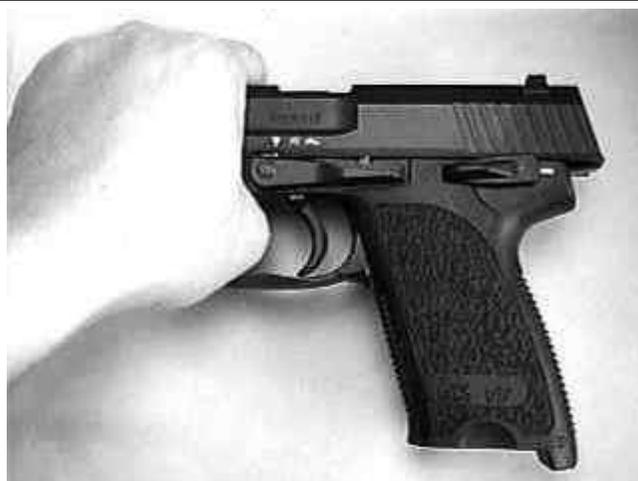
**Detail of Slide being held in "aligned" position**
