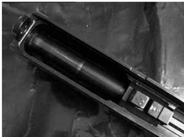
Barrel during removal
