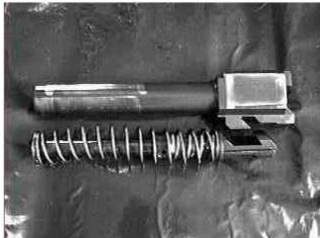
**Correct Barrel to Recoil/Buffer Spring Assembly Orientation**
