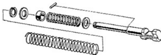
**Exploded View of the Recoil/Buffer Spring Assembly**
