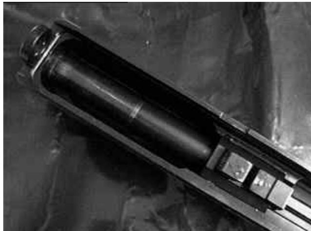
**Detail of Barrel in assembled position**
