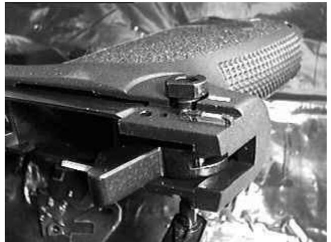
**Hammer Axle partially removed
