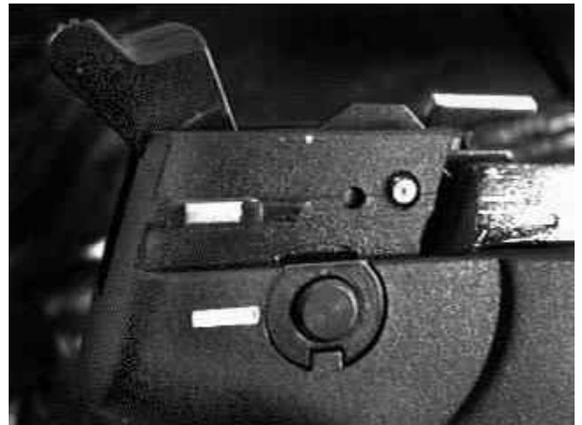
**Detail of right side of Frame showing Sear Axle in final position**
