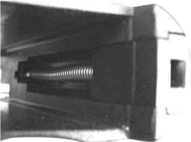
**Detail viewed inside Magazine Well showing Hammer Spring correctly aligned with the Lanyard Loop Insert**
