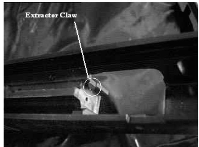
**Extractor Claw and Firing Pin Hole area**
