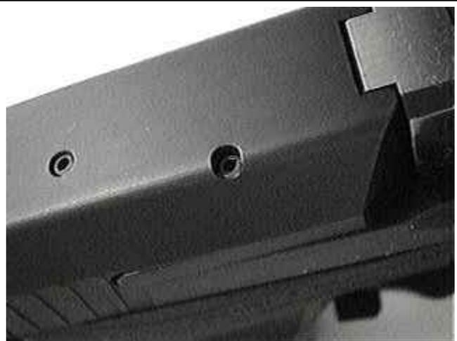
**Extractor and Firing Pin retainer Roll Pins**
