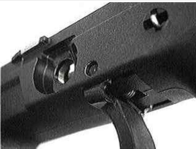
**Detail of Trigger, Spring, and Axle viewed from below
