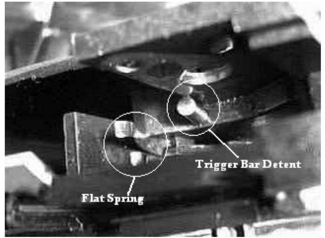
**Detail view of the Flat Spring (left) and the Trigger Bar Detent (right)**
