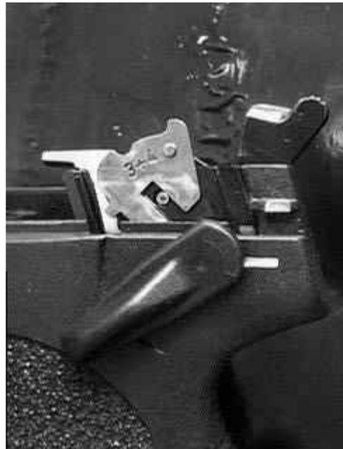
**Detail of the Detent Plate during installation (note the Sear Axle end is flush with the left wall of the Frame)**
