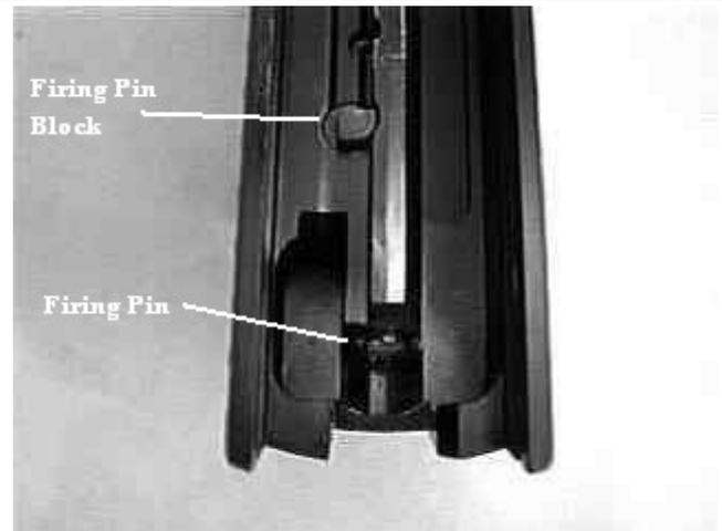
**Rear view of Firing Pin Block (top)
