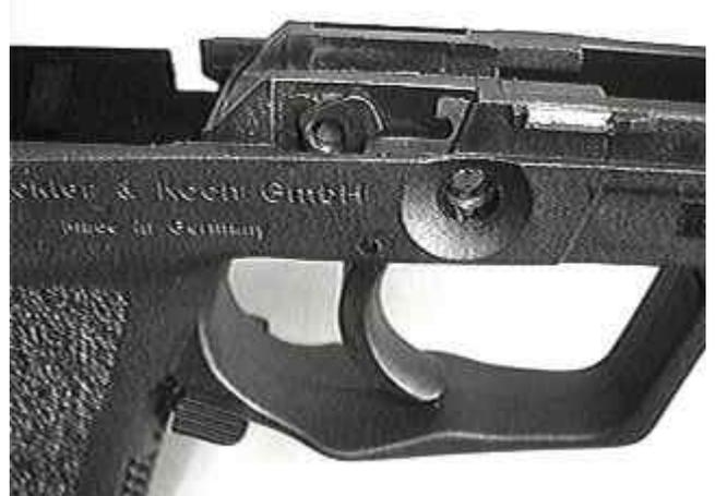
**Detail of Trigger pivot point after Trigger Bar is removed**
