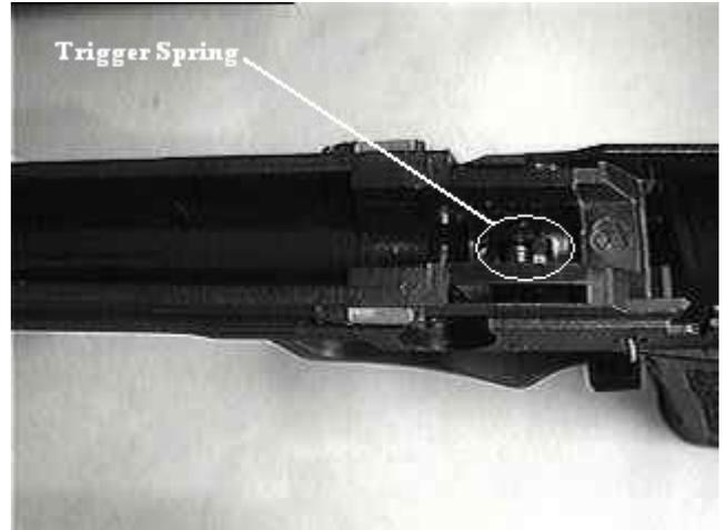
**Detail of Frame and Trigger Spring area & area normally under the Slide**
