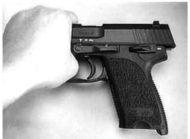
**Holding the Slide/Frame Assy. prior to Slide Release removal**
