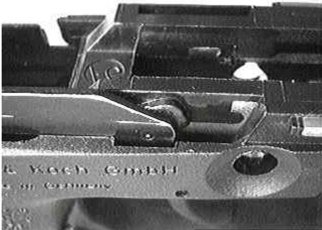
**Detail of Trigger to Trigger Bar pivot point**
