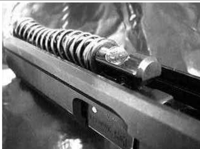
Recoil/Buffer Spring Assembly prior to removal
