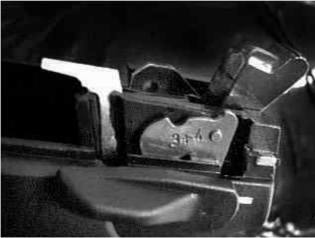
**Detail of detent Plate after engagement with Control Lever Axle (prior to pressing down against Detent Slide/Compression Spring)**
