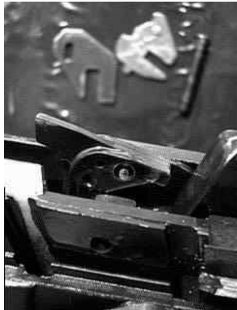
**Catch and Control Latch rotating up and back**
