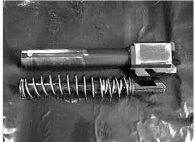
**Correct Barrel to Recoil/Buffer Spring Assembly orientation**
