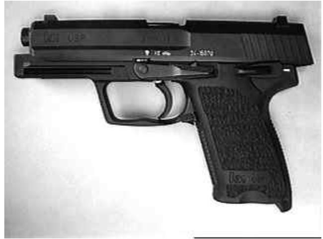
**Detail of Slide Notch aligned and Slide Release partially inserted.**
