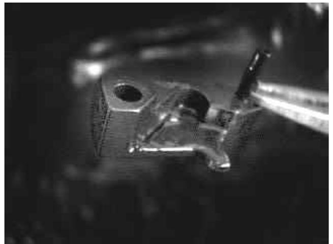
**Detail of the Sear (the pin end is inserted downward between the Flat Spring and the Hammer)**
