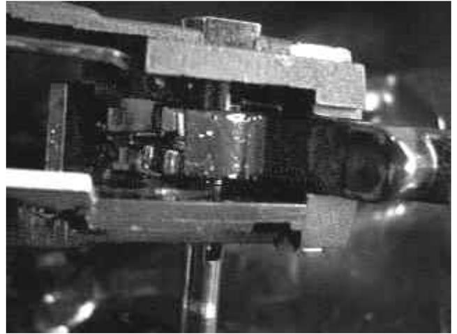
**Detail of Hammer with Hammer Axle partially installed (Control Lever not yet fully inserted)**
