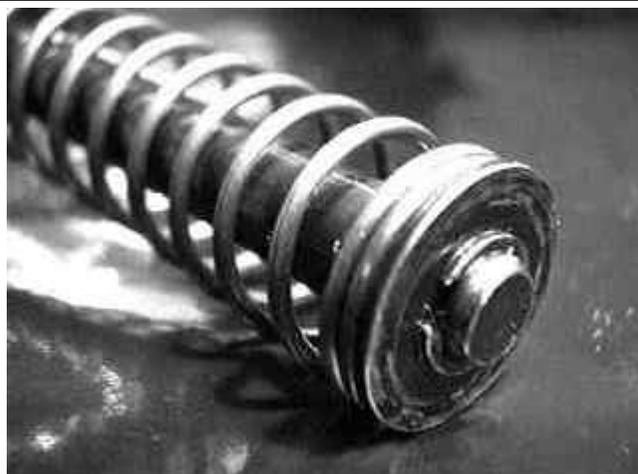
Detail of Guide Rod end, Spring, Retainer, and Snap-Ring on "captured" Recoil/Buffer Spring Assembly
