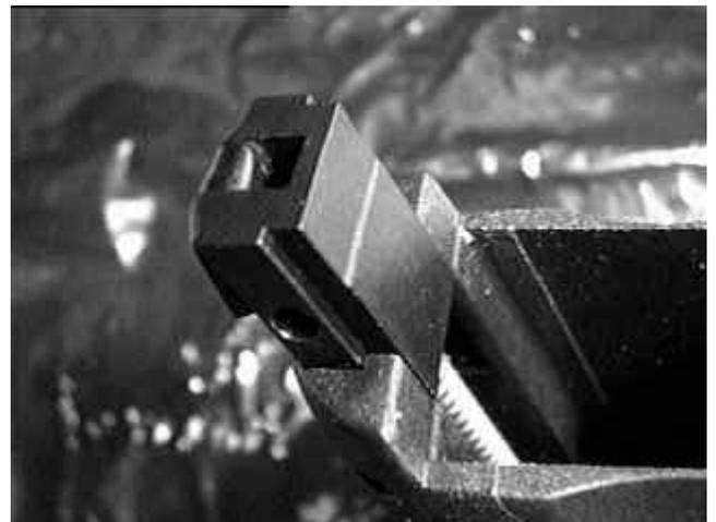
**Lanyard Loop Insert with Pin removed**
