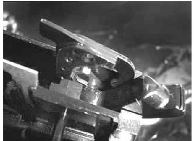
**Detail of the Catch (left) and Control Latch (right) Assembly before final installation**
