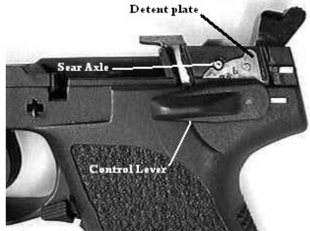
**Left side of frame, showing the control detent plate**
