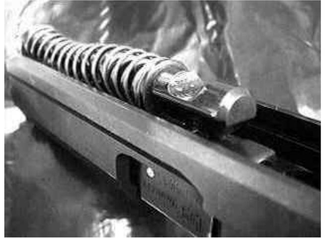
**Recoil/Buffer Spring Assembly engaged with Locking Block (final position)**
