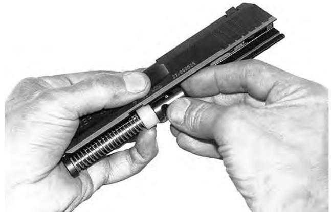
Insert the recoil spring guide rod
