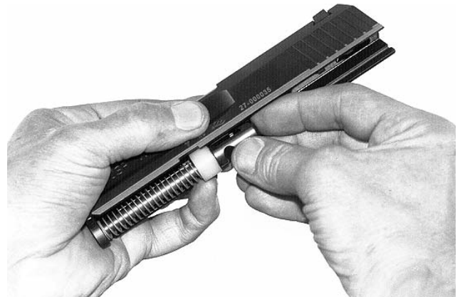
Insert the recoil spring guide rod
