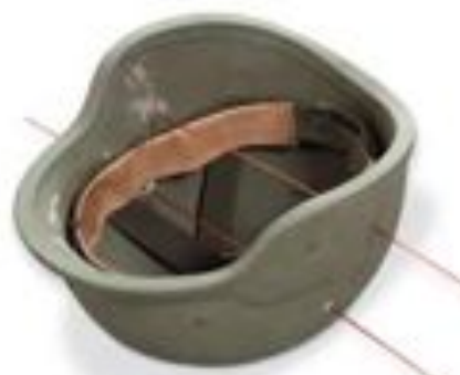
Kevlar helmet penetration at 200 meters. The same 4.6 mm cartridge easily passes through automobile windshields with minimal deflection.
