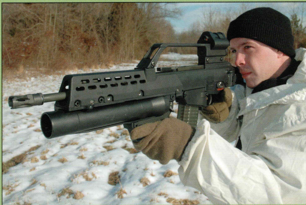
AG-36 attached to the G36 rifle as used by the German military.
